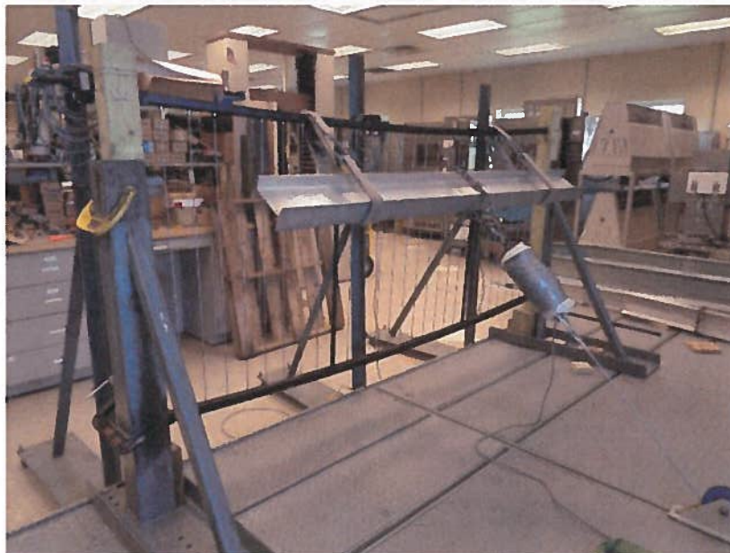
Photo No. 6 Uniform Load at 45 degrees from Horizontal on Top Rail
