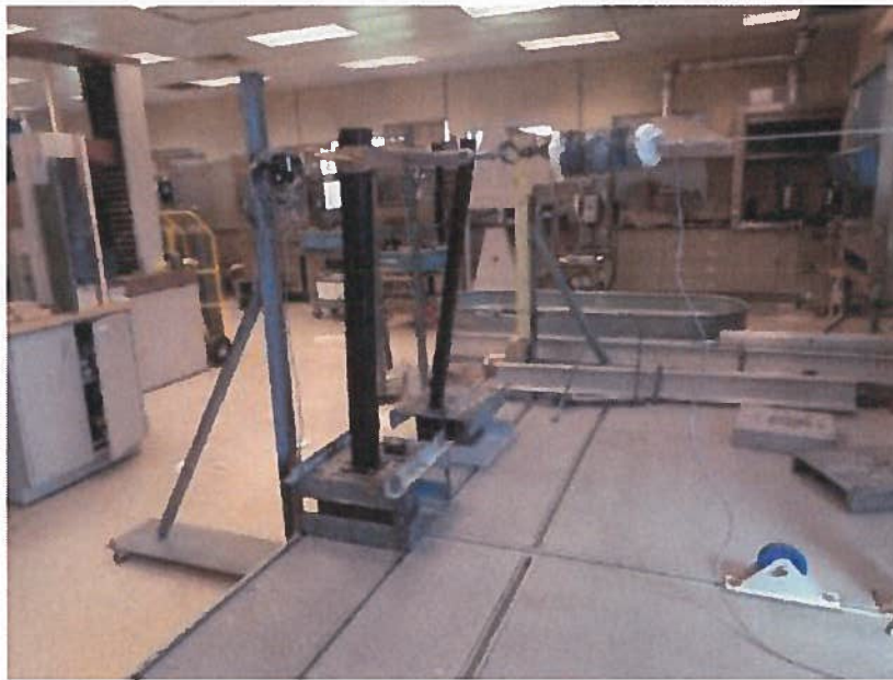
Photo No. 9 Concentrated Load Test at Top of Post Mount
