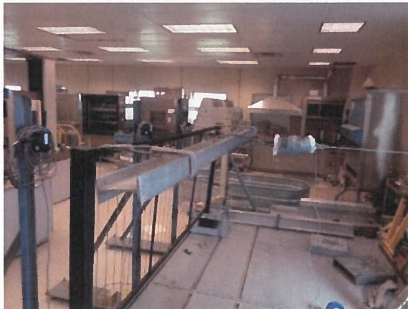
Photo No. 8 Concentrated Load at Ends of Top Rail (Brackets)
