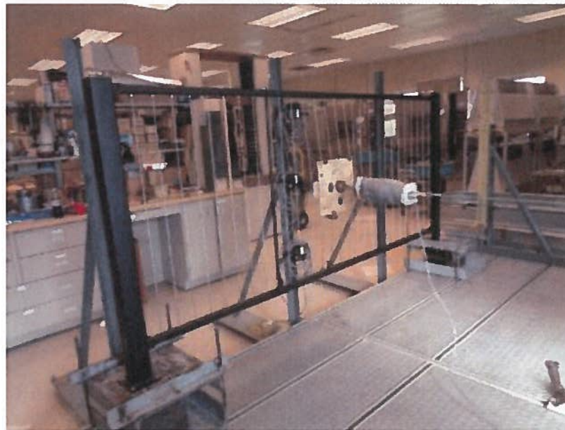
Photo No. 2 In-Fill Load Test at Center of Cable Infill
