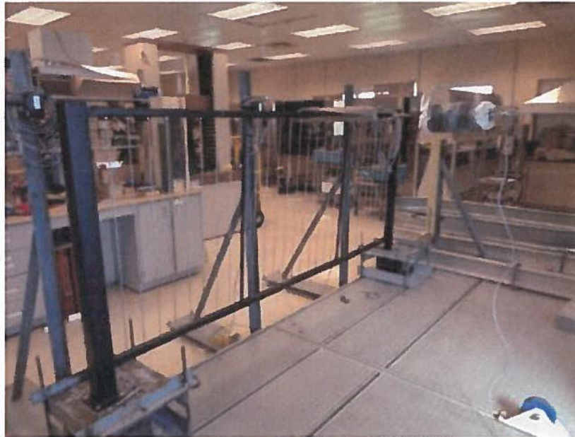
Photo No. 7 Concentrated Load Test at Mid-Span of Top Rail
