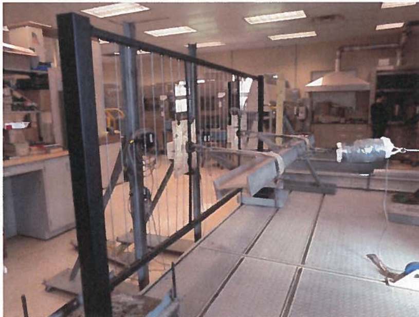
Photo No. 4 In-Fill Load Test at Center of Two Intermediate Pickets
