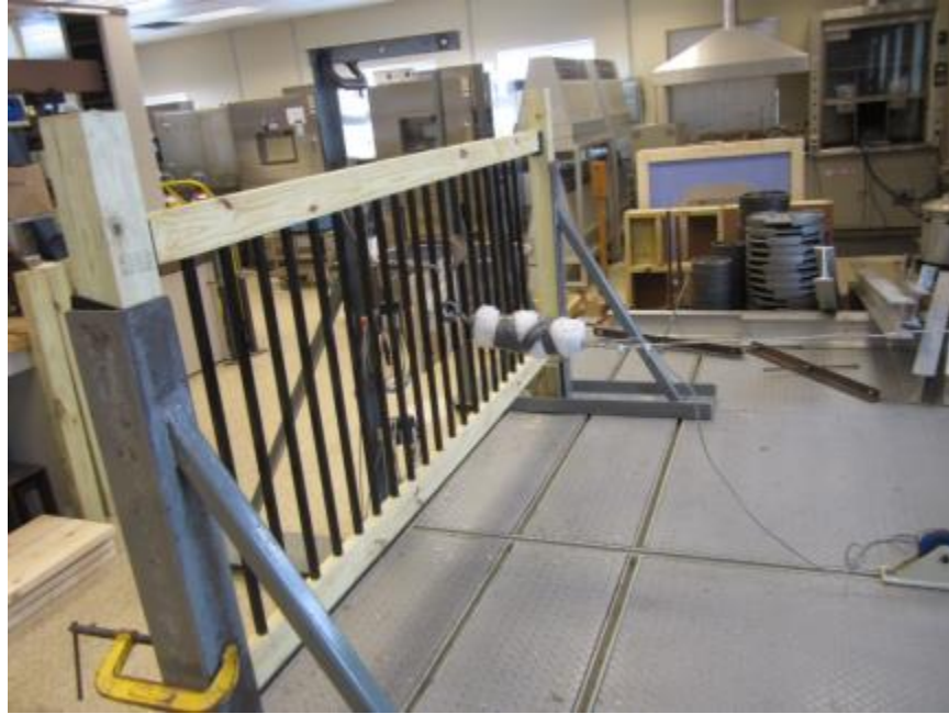
Photo No. 1 Infill Loading at Center of Three Balusters
