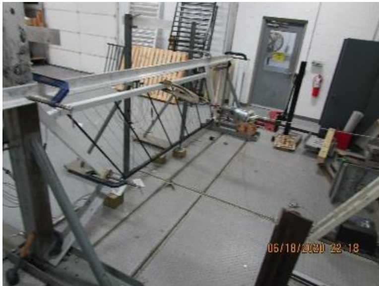
Photo No. 6 Horizontal Concentrated Load Test at Midspan of Top Rail (Cable Infill and Glass Balusters)
