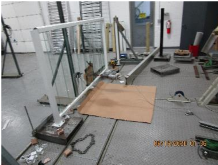
Photo No. 2 In-Fill Load Test at Bottom of Glass Baluster Infill
