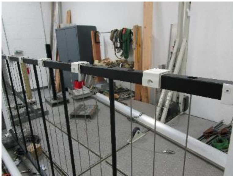
Photo No. 12 Intermittent Spacers
