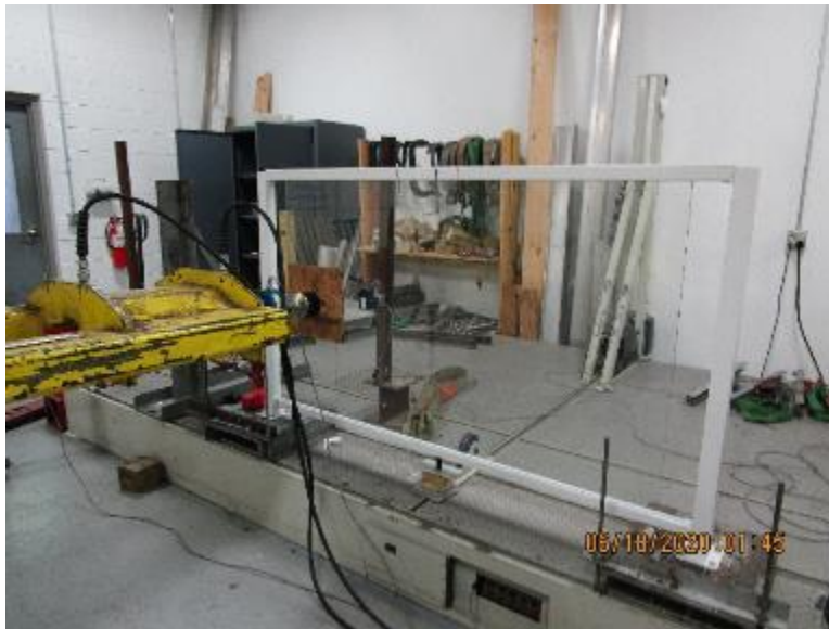
Photo No. 5 In-Fill Load Test at Edge of Glass Panel
