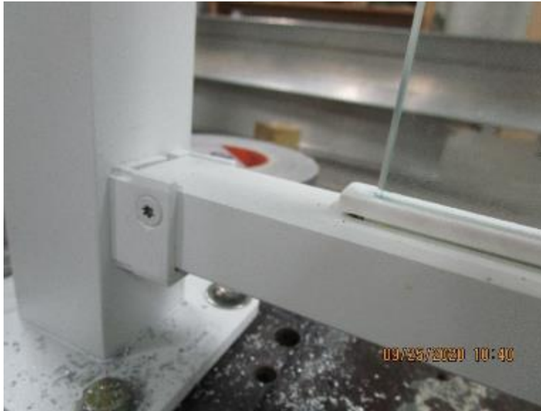
Photo No. 9 Cast Aluminum Level Rail Bracket
