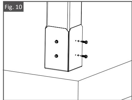
**Connection 2: Post To Double Beam Joist**
