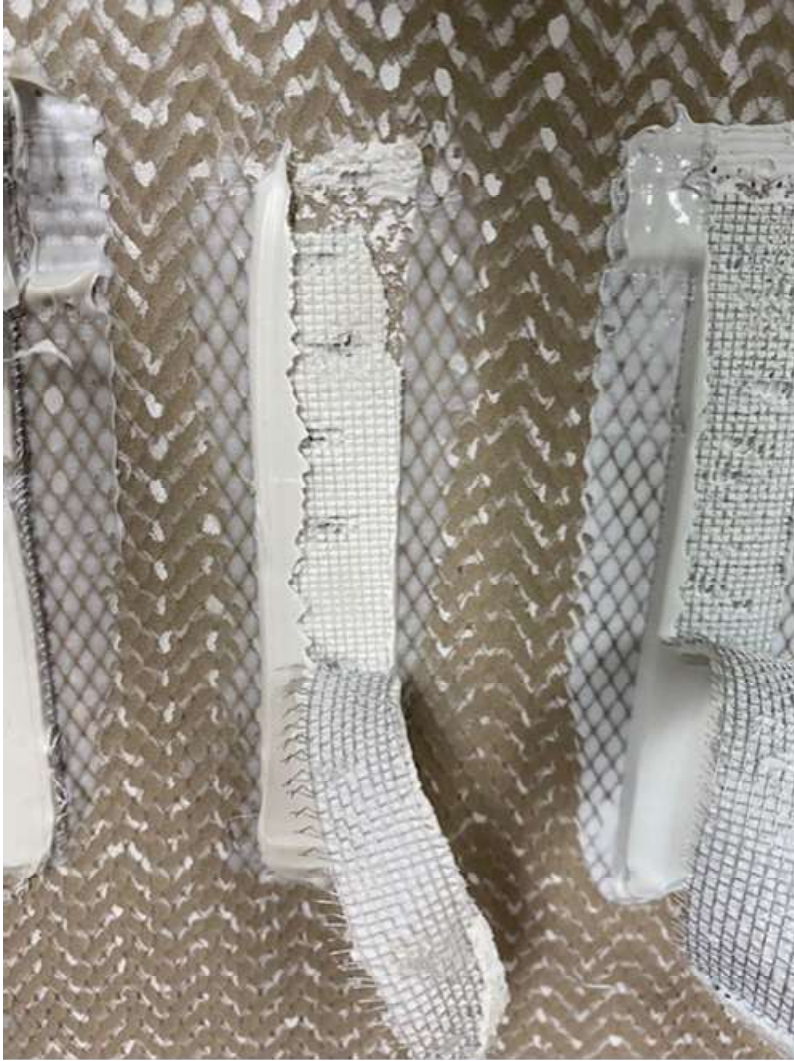
Fig 5. Post test: Picture showing cohesive failure for Titegrab on outdoor tile. Good adhesion to the outdoor tile.
