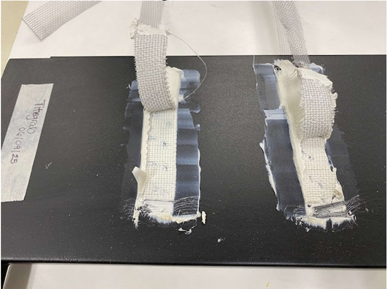
Fig 3. Post test: Picture showing cohesive failure for Titegrab on steel deck frame. Good adhesion to the frame.
