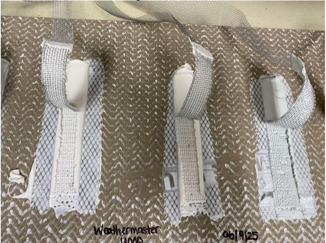
Fig 4. Post test: Picture showing cohesive failure for Weathermaster on outdoor tile. Good adhesion to the outdoor tile.
