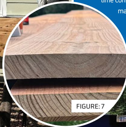
Figure 7: Warping and crowning naturally occurring.
