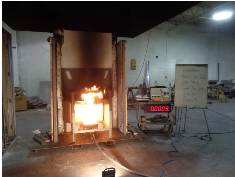
Photo No. 5 Ignition of Burner
