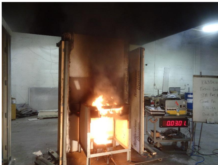
Photo No. 6 Ignition on Top of Deck
