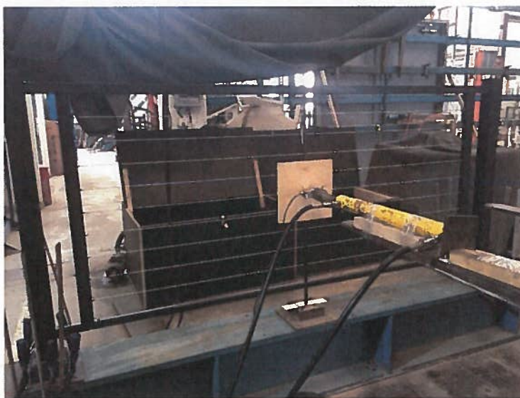
Photo No. 3 In-Fill Load Test at Center of Two Pickets
