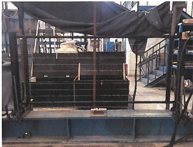
Photo No. 8 Concentrated load on post horizontally
