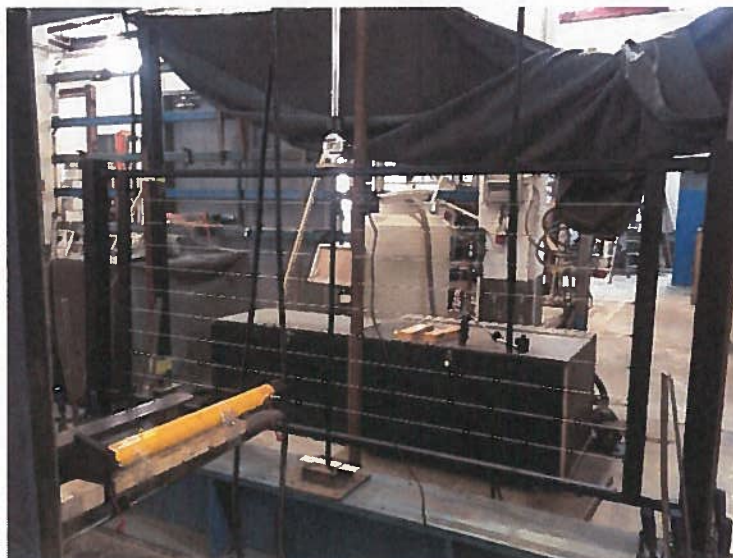
Photo No. 4 Concentrated load on mid top rail vertically
