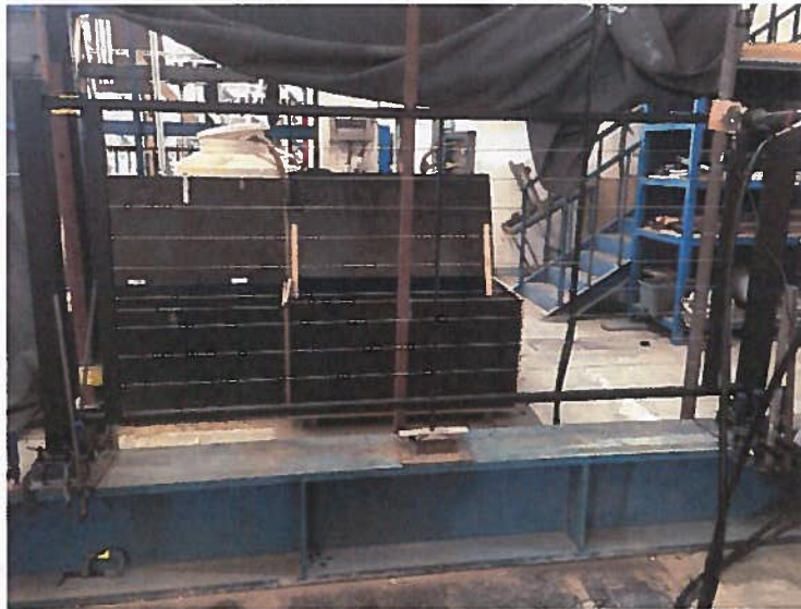
Photo No. 7 Concentrated load on top bracket horizontally
