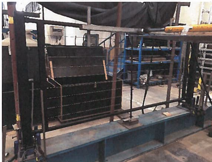
Photo No. 10 Uniform load horizontally
