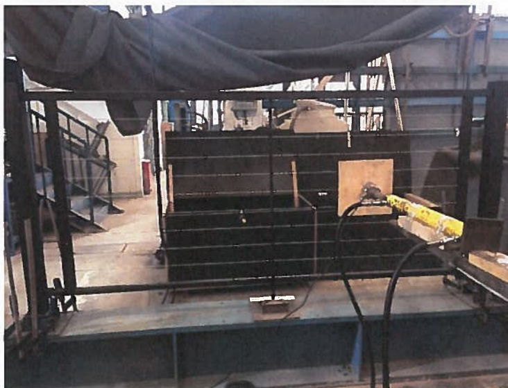
Photo No. 2 In-Fill Load Test at Center of half panel
