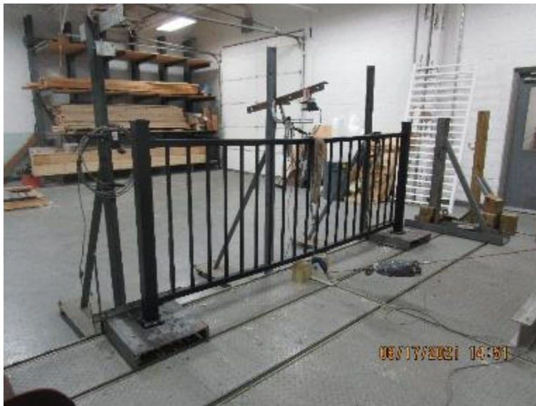
Photo No. 4 Vertical Concentrated Load Test at Midspan of Top Rail
