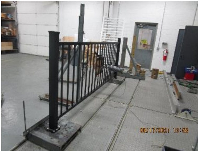
Photo No. 1 In-Fill Load Test at Center of Two Pickets
