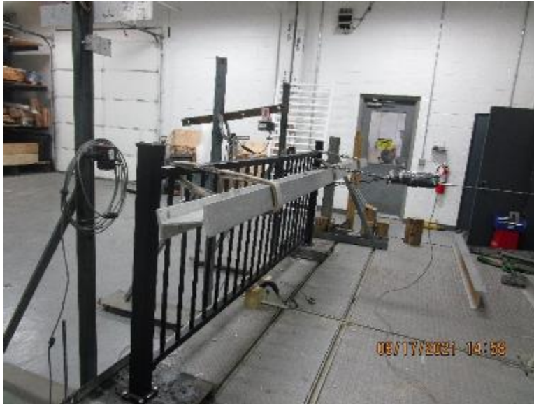
Photo No. 5 Concentrated Load Test at Ends of Top Rail (Brackets)
