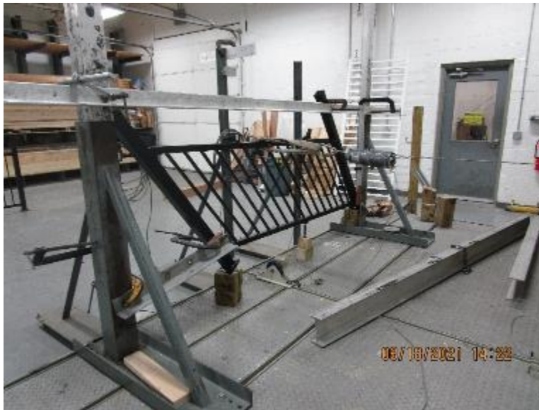
Photo No. 3 Horizontal Concentrated Load Test at Midspan of Top Rail
