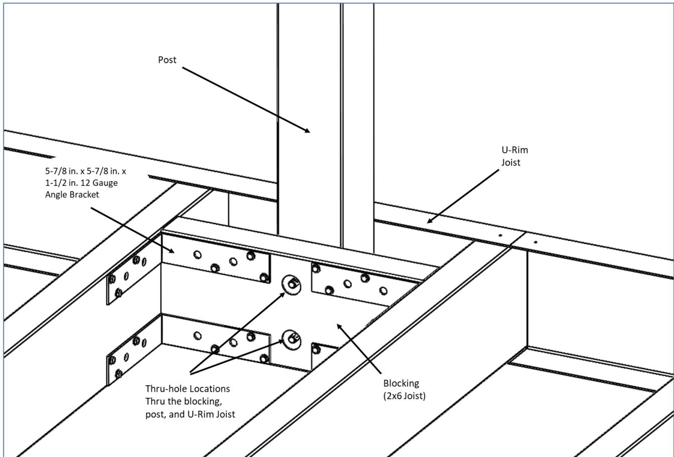
Cut blocking using the Evolution 2x6 Joist. Position and install blocking so the post will fit snug between the U-Rim Joist and the cut 2x6 blocking piece. Install with 5-7/8 in. x 5-7/8 in. x 1-1/2 in. 12 Gauge Angle Bracket using the Evolution Self-Drilling Screw.
