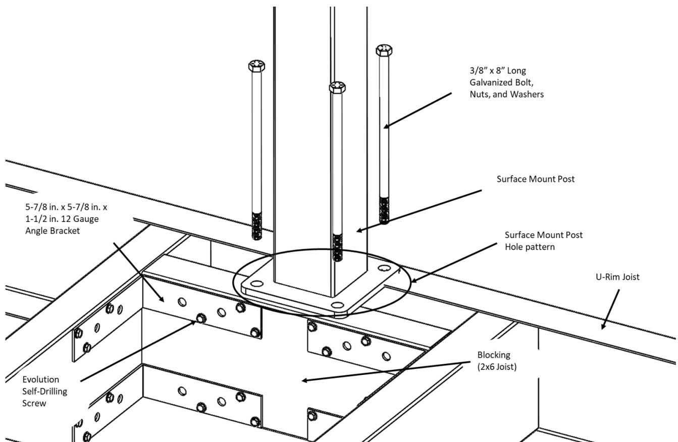
Cut blocking using the Evolution 2x6 Joist. Position and install blocking according to the required hole spacing of the surface mount post. Install with 5-7/8 in. x 5-7/8 in. x 1-1/2 in. 12 Gauge Angle Bracket using the Evolution Self-Drilling Screw.
