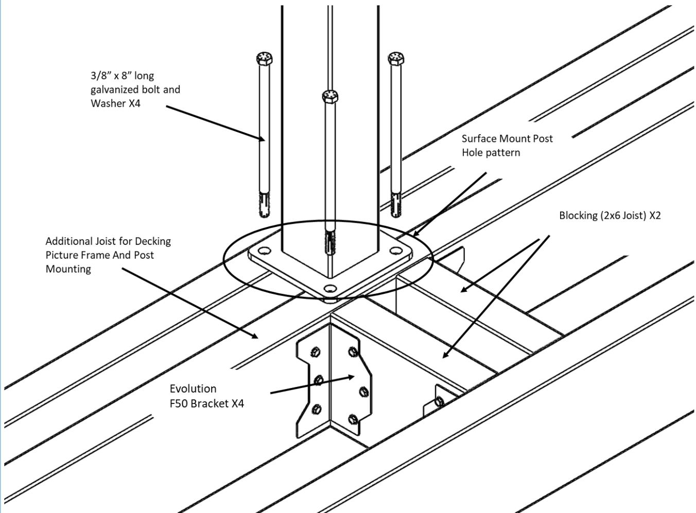
Cut (2) pieces of blocking using the Evolution 2x6 Joist. Position and install using (4) F50 brackets according to the required hole spacing of the surface mount post. Install with Evolution F50 Brackets using the Evolution Self-Drilling Screw.
