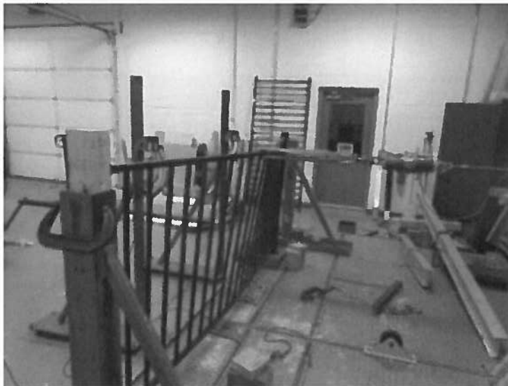
Photo No. 6 Concentrated Load Test at Mid-Span of Top Rail
