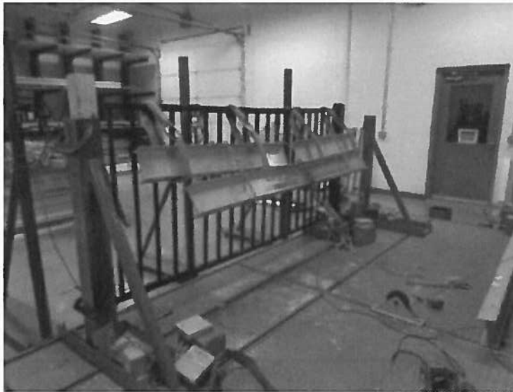
Photo No. 5 Uniform Load Applied at a 45 degree angle
