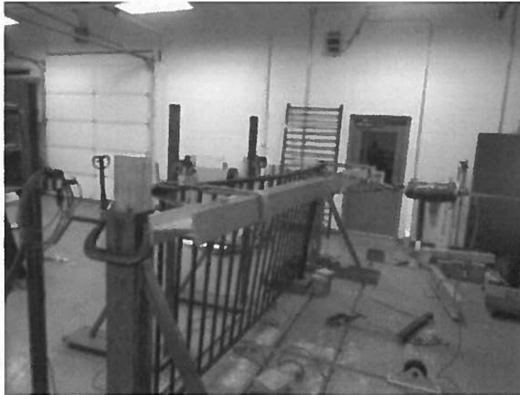
Photo No. 7 Concentrated Load Test at Ends of Top Rail (Brackets)
