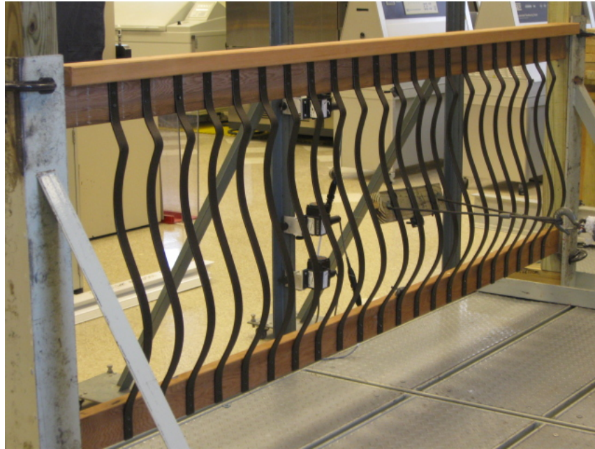
Photo No. 1 In-Fill Load Test at Center of Three Vienna Series Balusters
