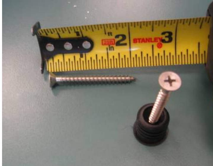
Photo No. 9 Nylon EZ Mounts for Attachment of Vintage Series Round Style Balusters to Rails
