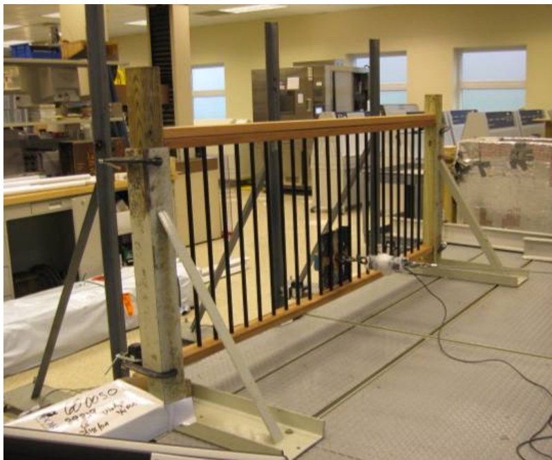
Photo No. 8 In-Fill Load Test at Bottom of Three Vintage Series Round Style Balusters (Installed with EZ Mounts)
