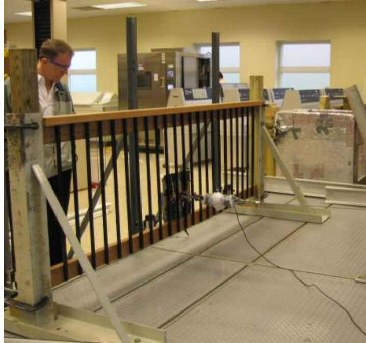
Photo No. 5 In-Fill Load Test at Bottom of Three Vintage Series Square Style Balusters
