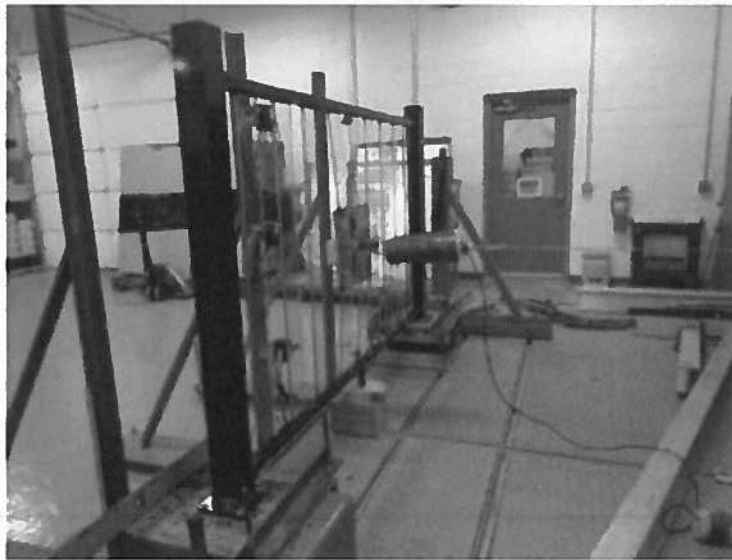
Photo No. 1 In-Fill Load Test at Center of Two Glass Balusters
