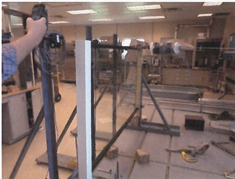
Photo No. 4 Horizontal Concentrated Load Test at Mid-Span of Top Rail
