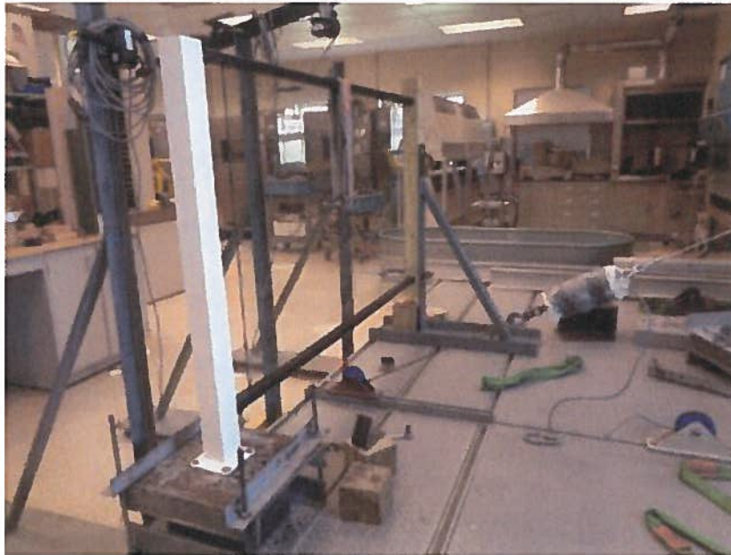
Photo No. 5 Vertical Concentrated Load Test at Top of Post Mount
