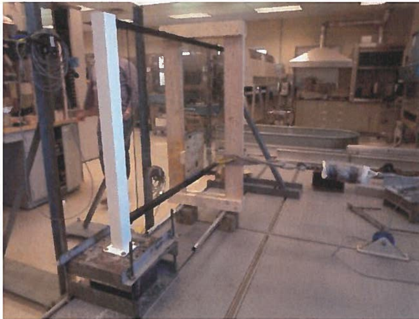
Photo No. 3 In-Fill Load Test at Bottom
