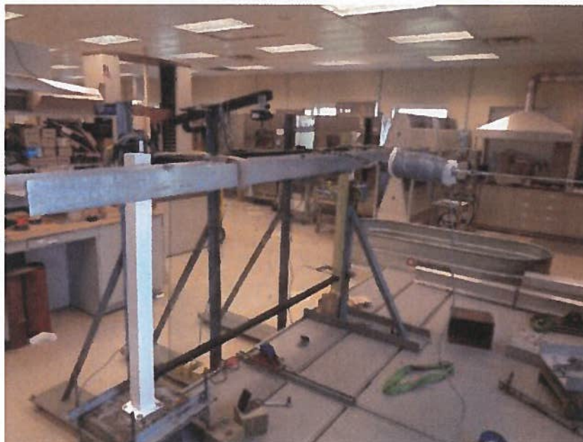
Photo No. 6 Concentrated Load at Both Ends of Top Rail (Brackets)
