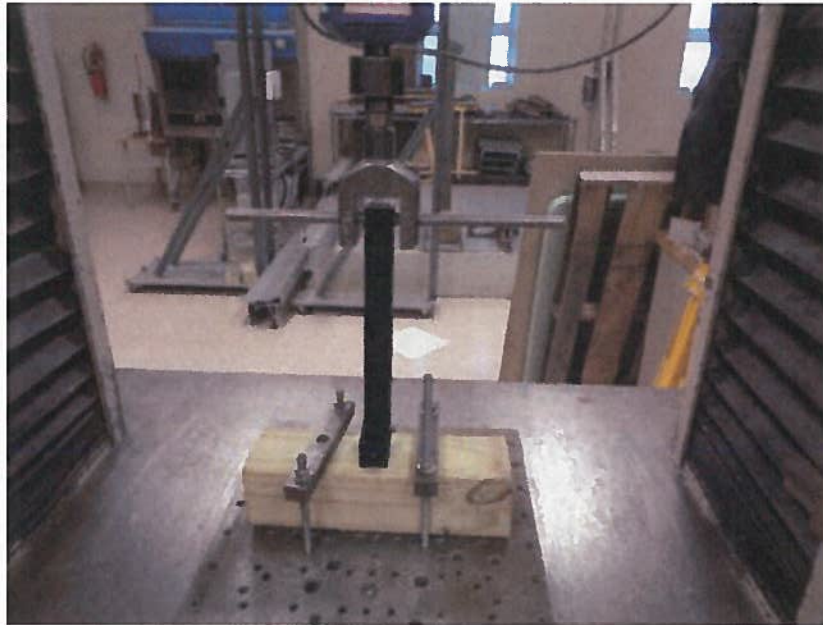
Photo No. 1 Assembly Fastener Test Setup
